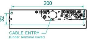
Step 1 – Fix Mounting Plate to Ceiling
